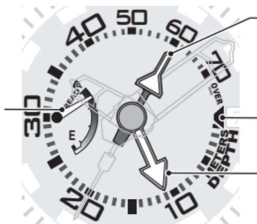
**Maximum water depth hand:** indicates the maximum depth during a measurement.
