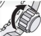
Push the crown in to the case. With gentle pressure towards the case, rotate the crown clockwise to secure it to the case. Be sure to tighten firmly. |
