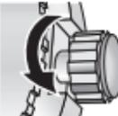
Rotate the locking screw counterclockwise, and loosen until it stops. |
