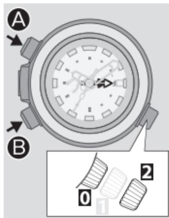
**5 Press and release the lower left button **B** to change the hand to be corrected.**
