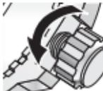
Rotate the crown counterclockwise until it releases from the case.    |
