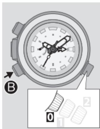
**1 Press and release the lower left button **B** while the crown's position is **0**.**
