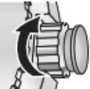
Rotate the locking screw clockwise, and tighten firmly.                                                                                               |
